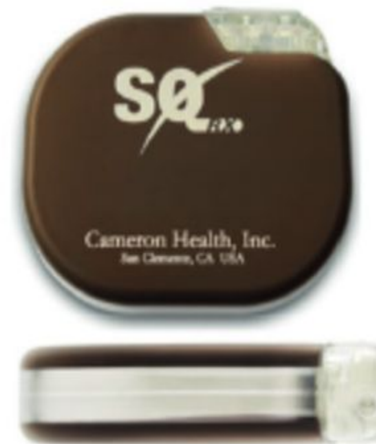
First-generation S-ICD SQ-RX 1010 (Cameron Health)
