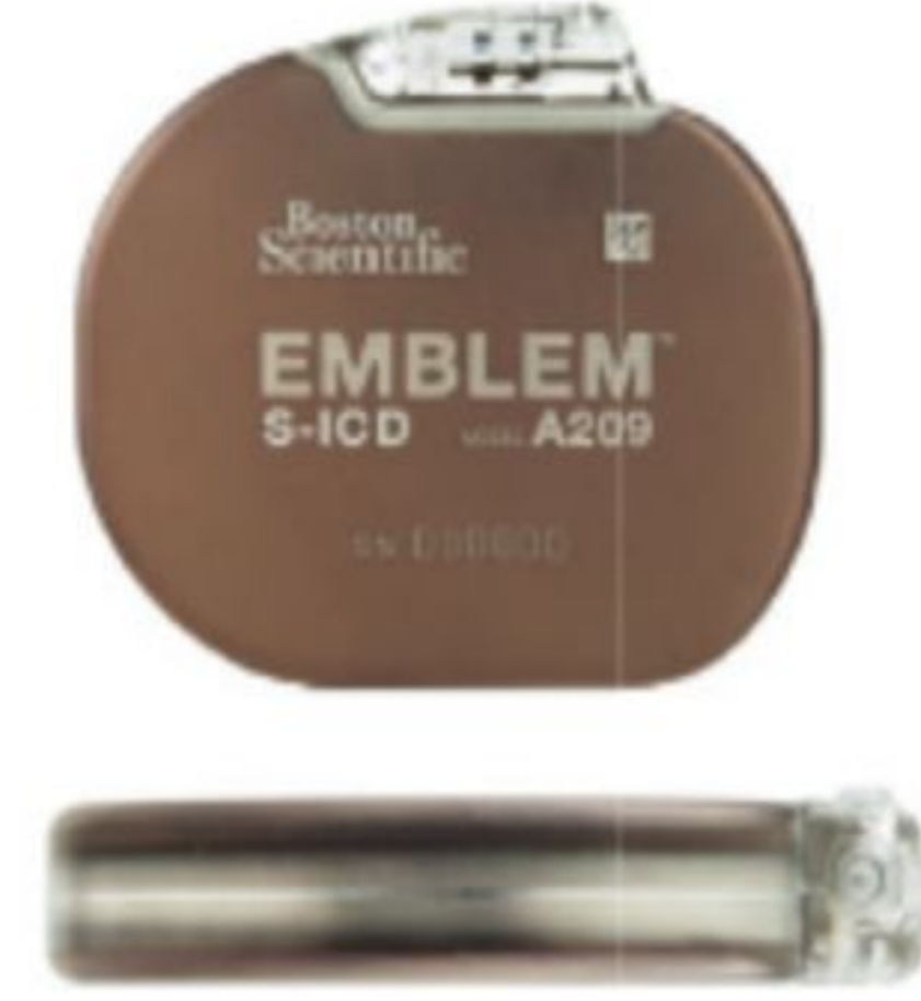
Second-generation S-ICD EMBLEM (Boston Scientific)
